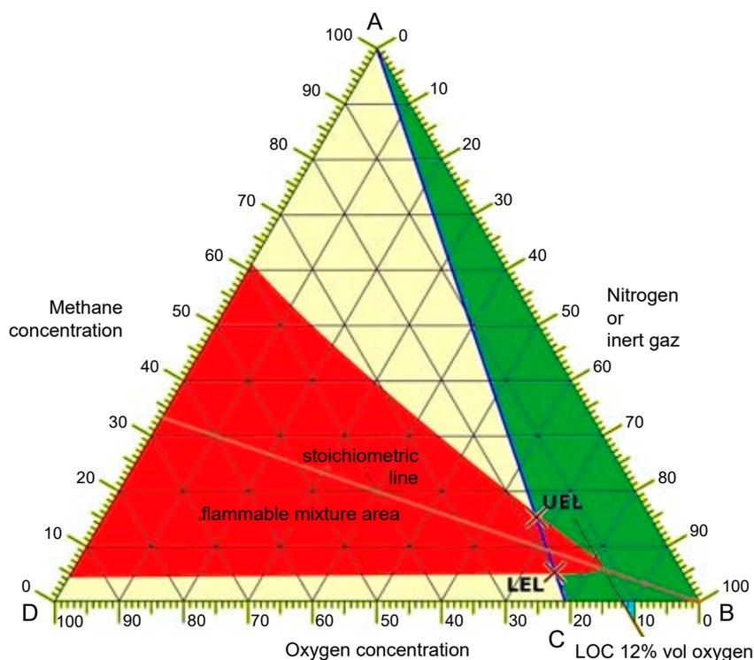
Figure 1. Diagram of methane-oxygen-inert gas mixtures
