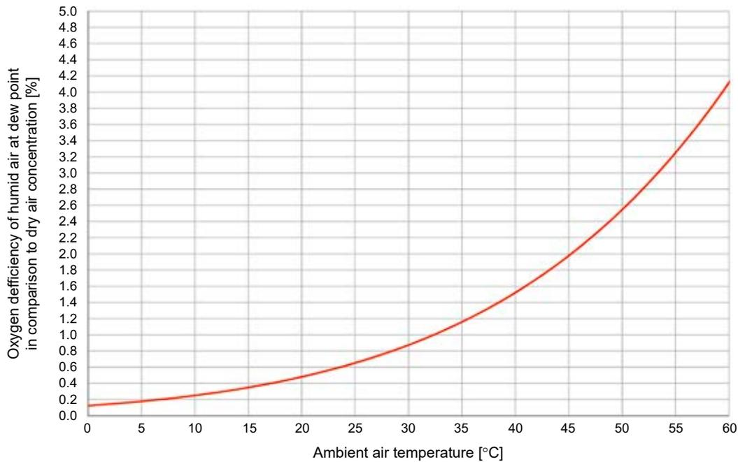
Figure 4. The oxygen deficiency in saturated air (at dew point) at pressure 101,325 Pa depending on ambient air temperature
