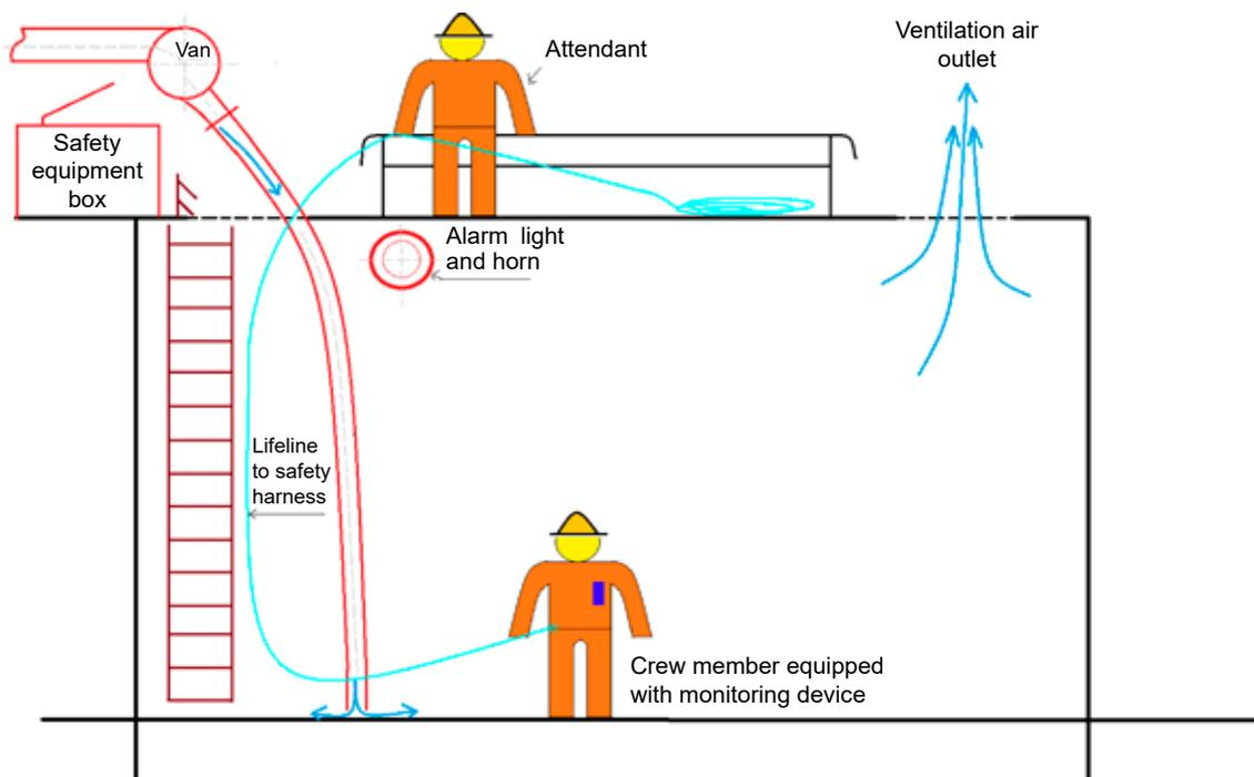
Figure 5. Essential conditions for allowing the work into enclosed spaces – the safety system
