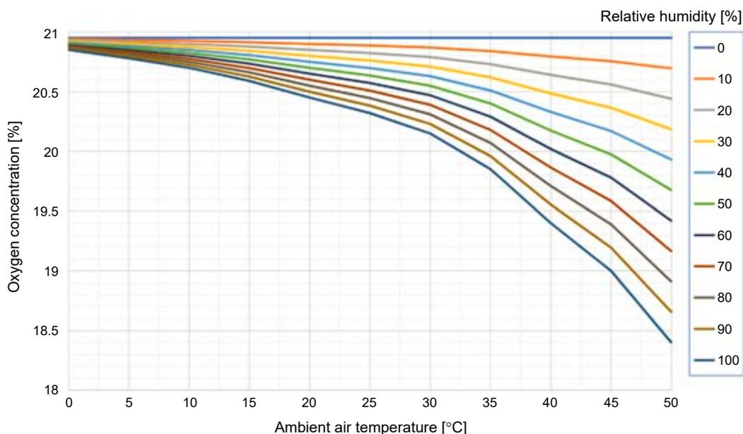
**Figure 2. The influence of air humidity on the volume (mole) concentration of oxygen depending on ambient temperature at air pressure 101,325 Pa**
