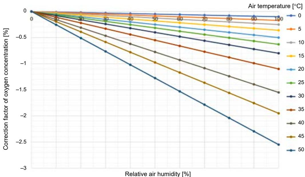
Figure 3. The influence of air temperature on the volume (mole) concentration of oxygen depending on humidity at air pressure 101,325 Pa
