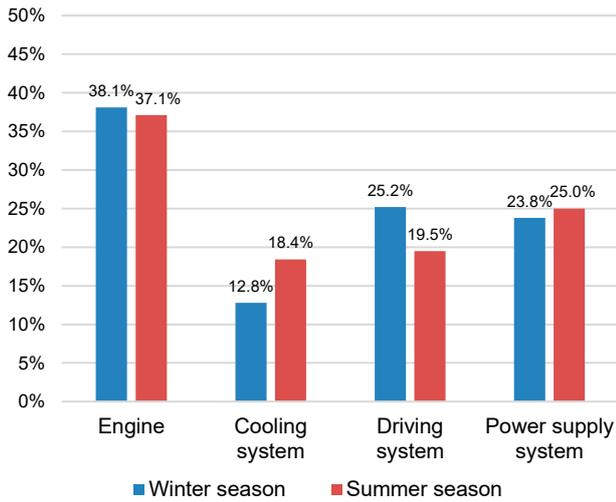
**Figure 3. Percentage of the occurrence of individual system failures depending on the annual season**
