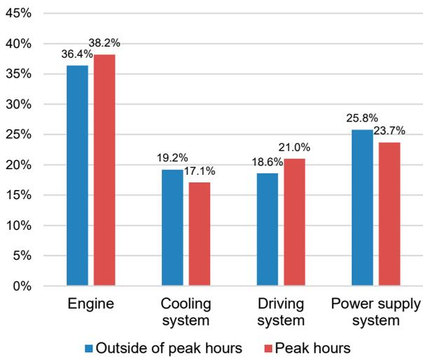
**Figure 4. Percentage of the occurrence of individual system failures depending on the peak hours in the summer season**
