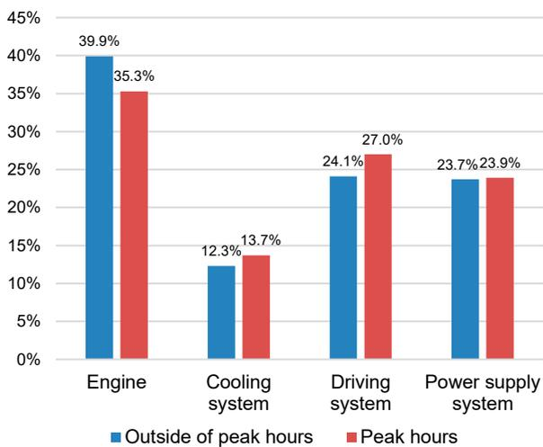
**Figure 5. Percentage of the occurrence of individual system failures depending on the peak hours in the winter season**
