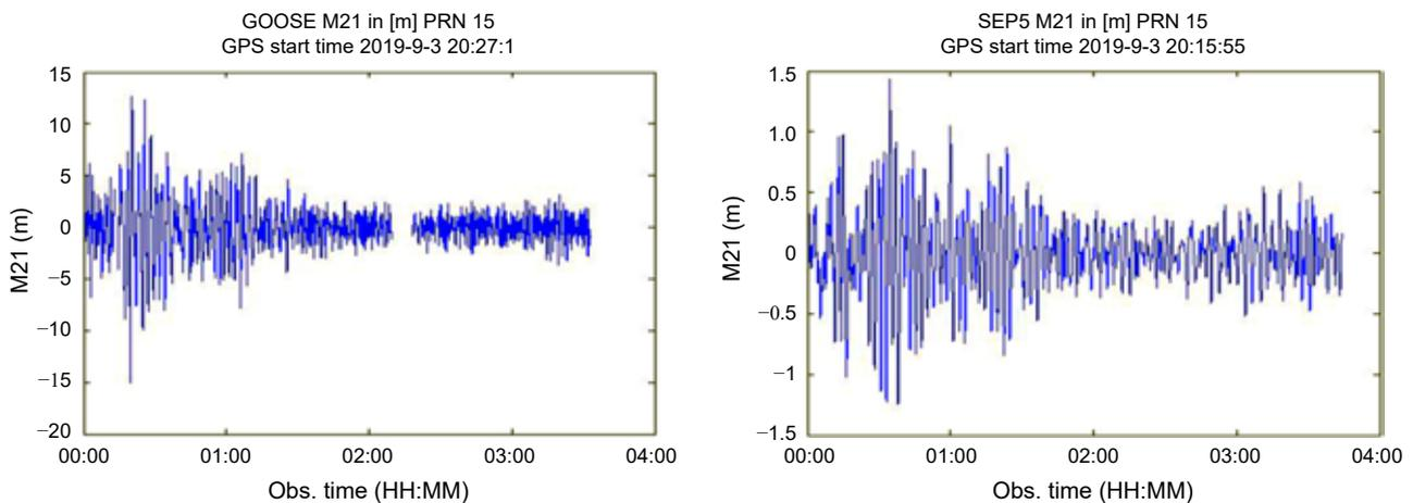
Figure 8. Example multipath plots (M21) of the GOOSE receiver (left) and the PolaRx5S receiver (right)
