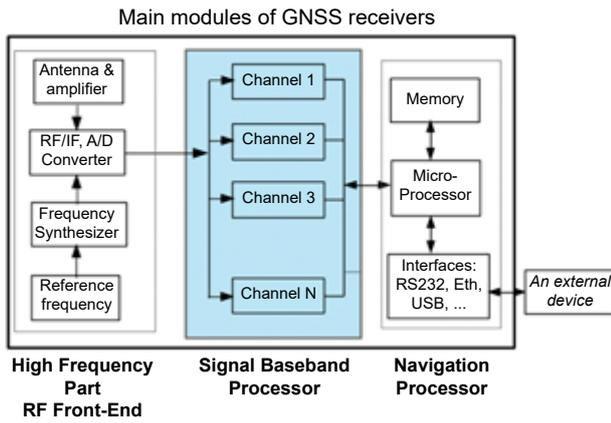
Figure 1. The architecture of GPS/GNSS standard receivers
