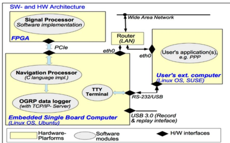
Figure 4. Software and hardware used in the testbed. User applications can also be run on the GOOSE embedded single-board computer
