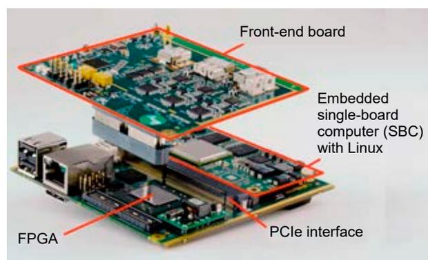
**Figure 3.** GOOSE Receiver in Single-Board Computer (SBC) configuration
