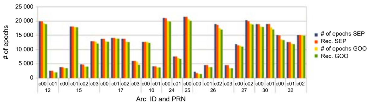
**Figure 6. Number of “nominal versus recorded” measurement-epochs for the selected GPS satellites**
