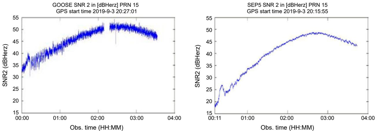
Figure 7. Signal-to-noise plots of the GOOSE receiver (left) and the PolaRx5S receiver (right)
