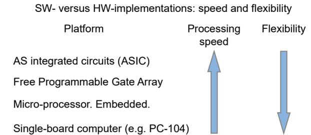
Figure 2. Comparison of the processing speed and flexibility of software- and hardware implementations
