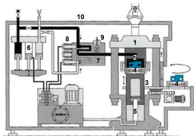
Figure 1. Design of the EXTRUDE HONE TEM P-350; 1 – Machine frame; 2 – Deburring Chamber; 3 – Index table; 4 – Closing plate; 5 – Closing hydraulic system; 6 – Gas metering system; 7 – Mixing block; 8 – Gas valves; 9 – Spark plug; 10 – Soundproof cabin; 11 – Index table rotating mechanism
