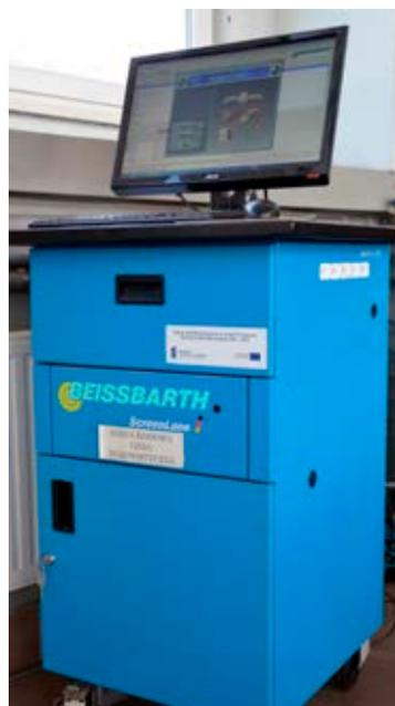
**Figure 2.** Control system of the Bosch Beissbarth SA 640 test stand
