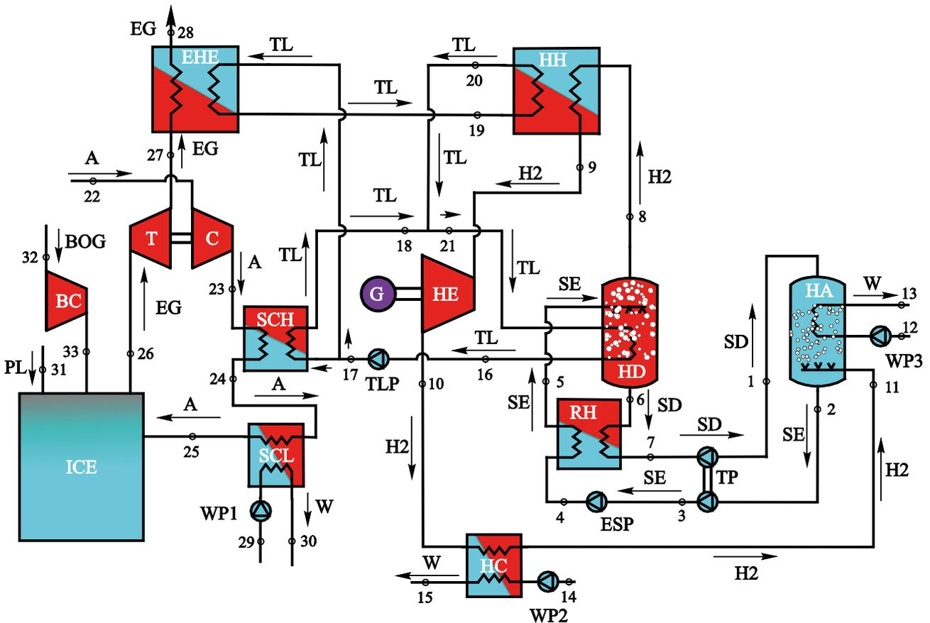
The numbers of control points (1 ... 33) corresponding to the temperatures ( $T_1 \dots T_{33}$ ), pressures ( $P_1 \dots P_{33}$ ), enthalpies ( $h_1 \dots h_{33}$ ), and heat flows (e.g.,  $Q_{1-2}$ ) considered in the text below.
