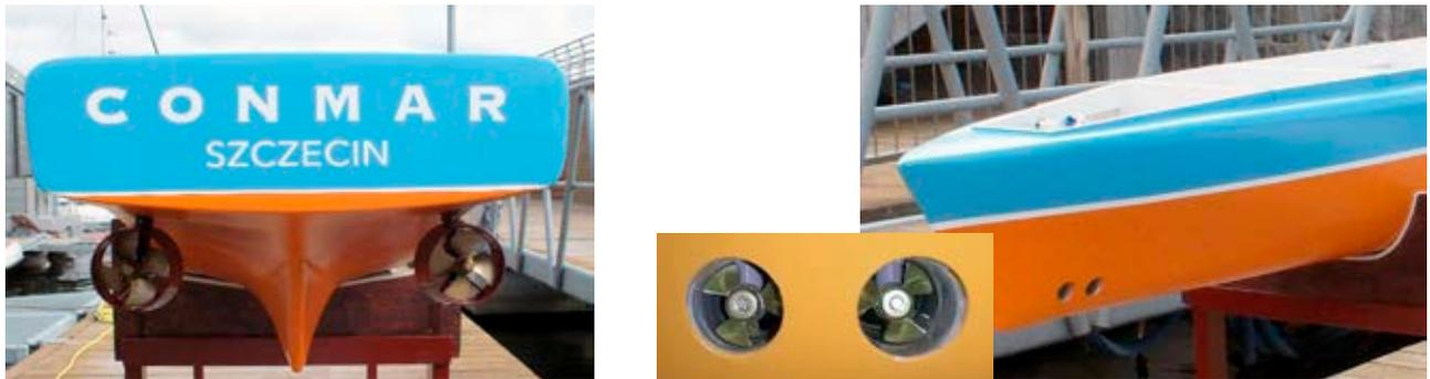
Figure 5. The propulsion system of the autonomous ship model
