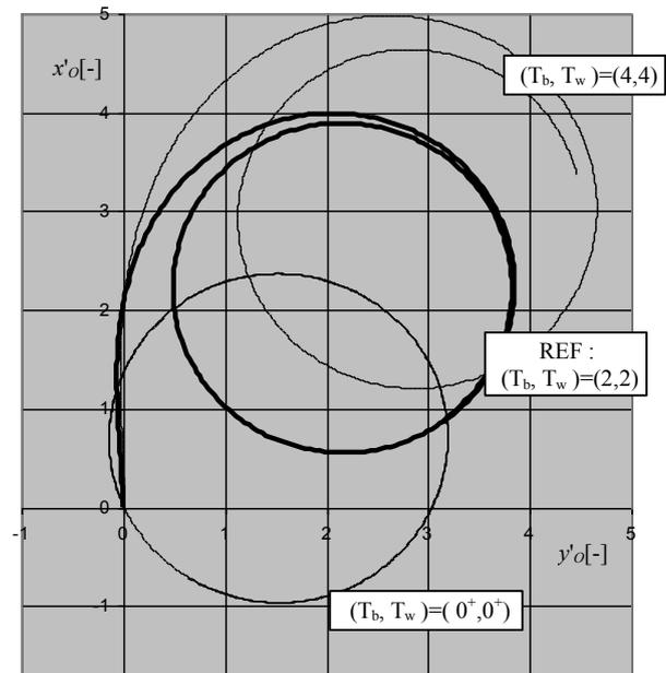
Fig. 4. The effect of equal yaw and drift time constants ( $T_b = T_w$ ) on trajectory
