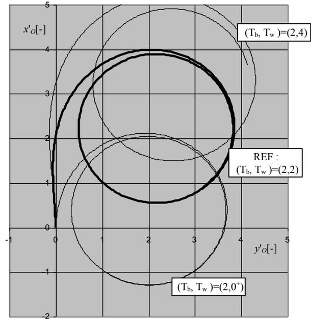
Fig. 3. The effect of yaw time constant  $T_w$  on trajectory
