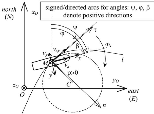
Fig. 1. Definition of ship kinematics
