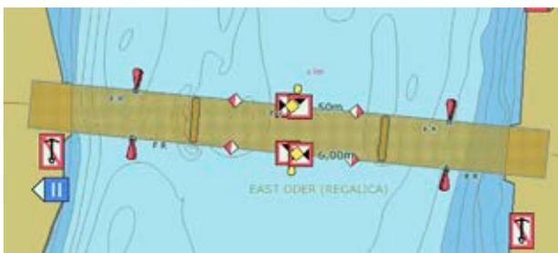
Figure 12. Mapped marks, lights, and span on the IENC map
