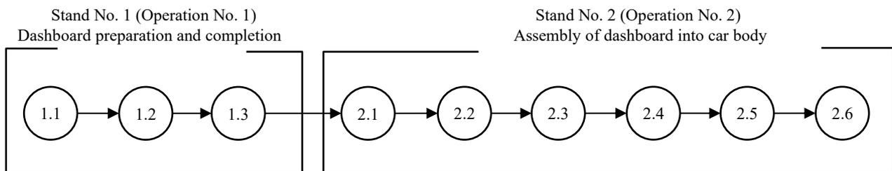
Figure 2. Graphic of the order of operations and tasks during the installation of the dashboard in the car body; operation numbers according to Table 1 (Ciszak, 2009)
