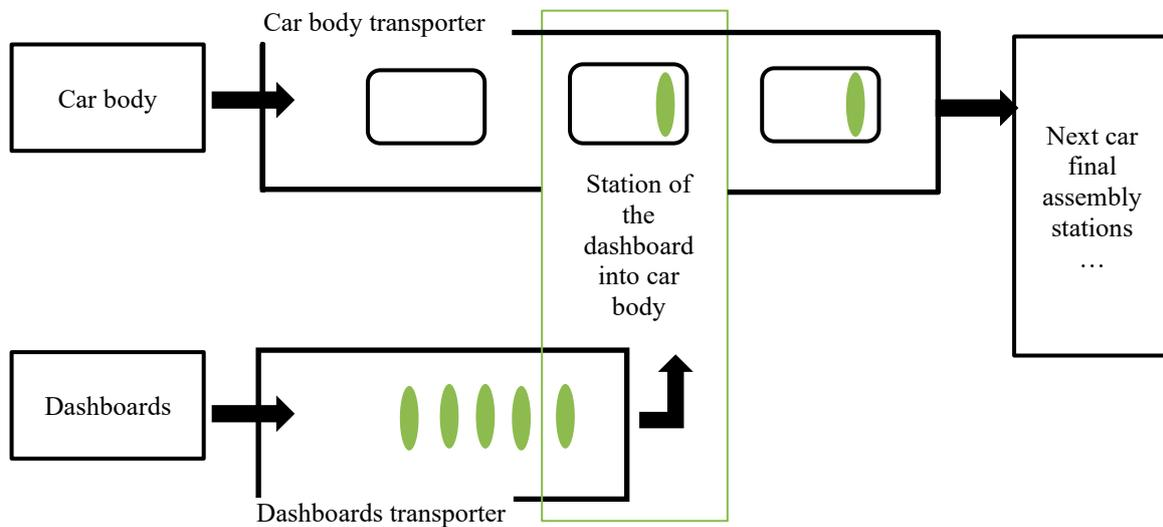
Figure 1. Organization chart of the dashboard installation site to the car body on the final assembly line (Ciszak, 2009)
