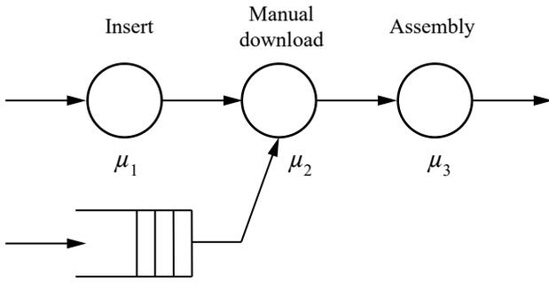
Figure 5. Queuing model for variant I of the production line
