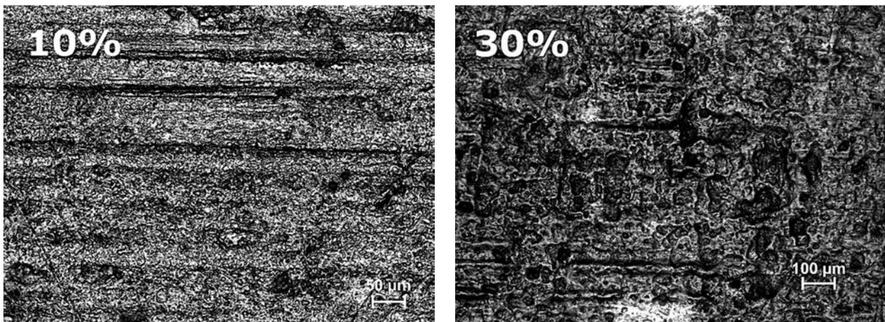
Figure 7. Cross section of the composite with 10% and 30% filler
