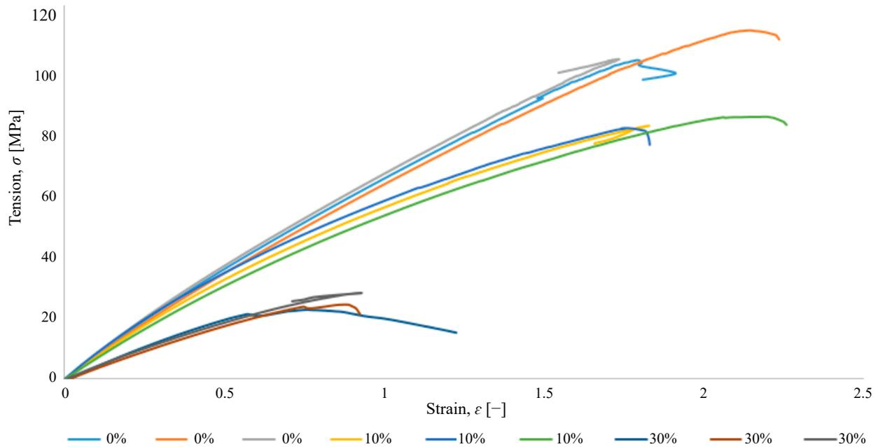
Figure 6. Static stretch test for samples with recyclate content of 0, 10, and 30%, with recyclate granulation  $\leq 1.2$  mm
