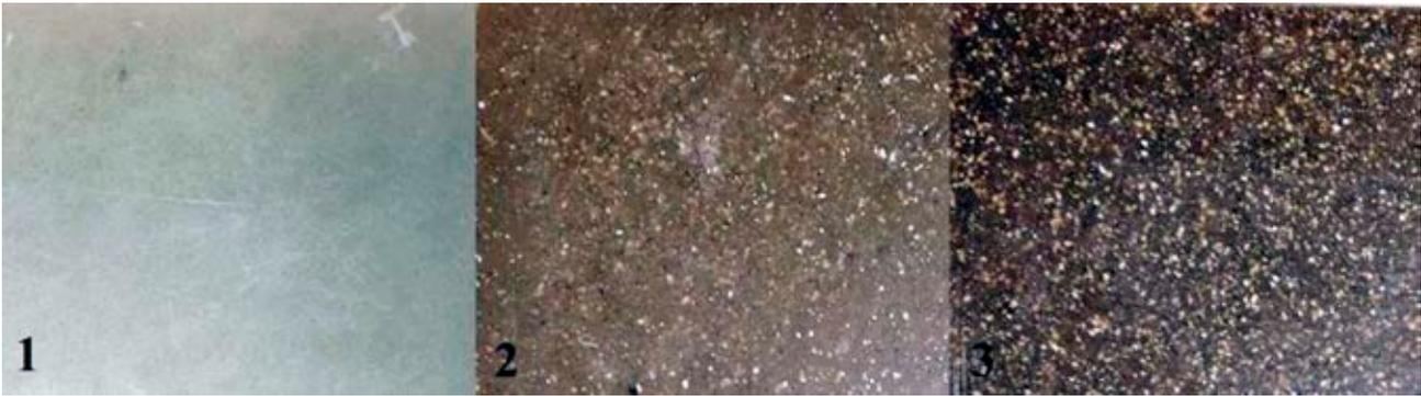
Figure 2. Hardened composite panels: 1 – without recyclate, 2 – 10% recyclate, 3 – 30% recyclate (photo taken with 13 Mpixel camera, Sony IMX 214 sensor and focal length 27 millimeters)
