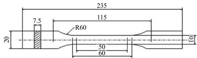
Figure 3. Dimensions of samples prepared for static stretching, according to standard PN-EN ISO 527-4\_2000P
