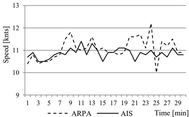
**Figure 8. Information on the true speed of the bulk carrier (38 767 GT) presented by AIS and ARPA installed on the bulk carrier “Magdalena Oldendorff”. Both ships were proceeding with steady courses and speeds in sea state 7 (Wilczyński, 2015)**
