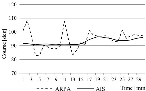
**Figure 4.** Information on the true course of the bulk carrier (40 500 GT) presented by AIS and ARPA installed on the LPG carrier “Pampero”. Both ships were proceeding with steady courses and speeds in sea state 3 (Wesołowski, 2016)
