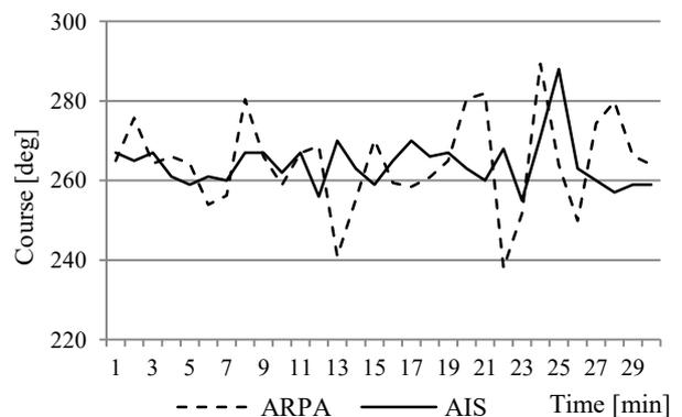
**Figure 7.** Information on the true course of the bulk carrier (38 767 GT) presented by AIS and ARPA installed on the bulk carrier “Magdalena Oldendorff”. Both ships were proceeding with steady courses and speeds in sea state 7 (Wilczyński, 2015)
