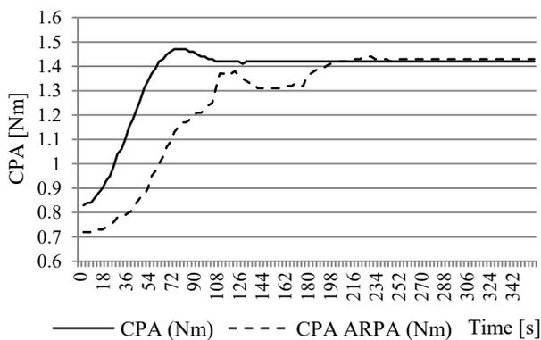
**Figure 9. Values of CPA indicated by ARPA (CPA ARPA) and simulated AIS (CPA) as the function of time in the measurement session 1**
