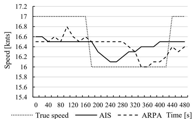
**Figure 14.** Values of true speed indicated by ARPA and AIS as a function of time for the test conducted on the Polaris simulator
