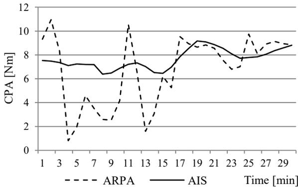
**Figure 3.** Information on the CPA of the bulk carrier (40 500 GT) presented by AIS and ARPA installed on the LPG carrier “Pampero”. Both ships were proceeding with steady courses and speeds in sea state 3 (Wesołowski, 2016)
