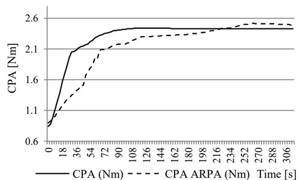
**Figure 11. Values of CPA indicated by ARPA (CPA ARPA) and simulated AIS (CPA) as the function of time in the measurement session 10**
