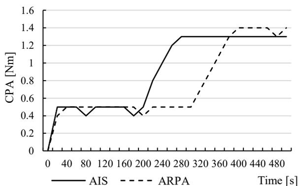
**Figure 12.** Values of CPA indicated by ARPA and AIS as a function of time for the test conducted on the Polaris simulator
