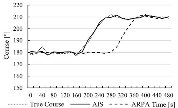
**Figure 13.** Values of true course indicated by ARPA and AIS as a function of time for the test conducted on the Polaris simulator
