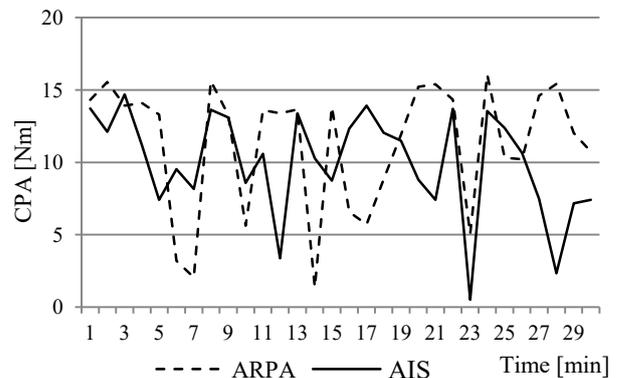
**Figure 6.** Information on the CPA of the bulk carrier (38 767 GT) presented by AIS and ARPA installed on the bulk carrier “Magdalena Oldendorff”. Both ships were proceeding with steady courses and speeds in sea state 7 (Wilczyński, 2015)
