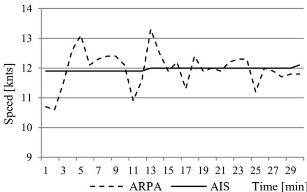
**Figure 5.** Information on the true speed of the bulk carrier (40 500 GT) presented by AIS and ARPA installed on the LPG carrier “Pampero”. Both ships were proceeding with steady courses and speeds in sea state 3 (Wesołowski, 2016)
