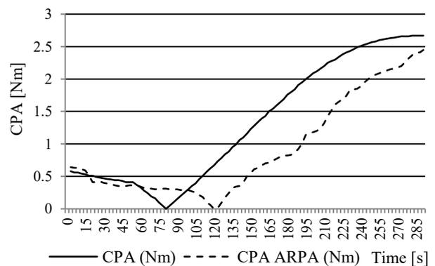
**Figure 10. Values of CPA indicated by ARPA (CPA ARPA) and simulated AIS (CPA) as the function of time in the measurement session 4**
