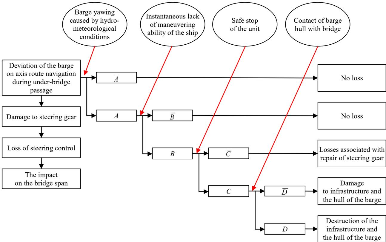
Figure 3. Model identification of risks during under-bridge passage of inland vessels, built with ETA techniques that take account of the probability of events
