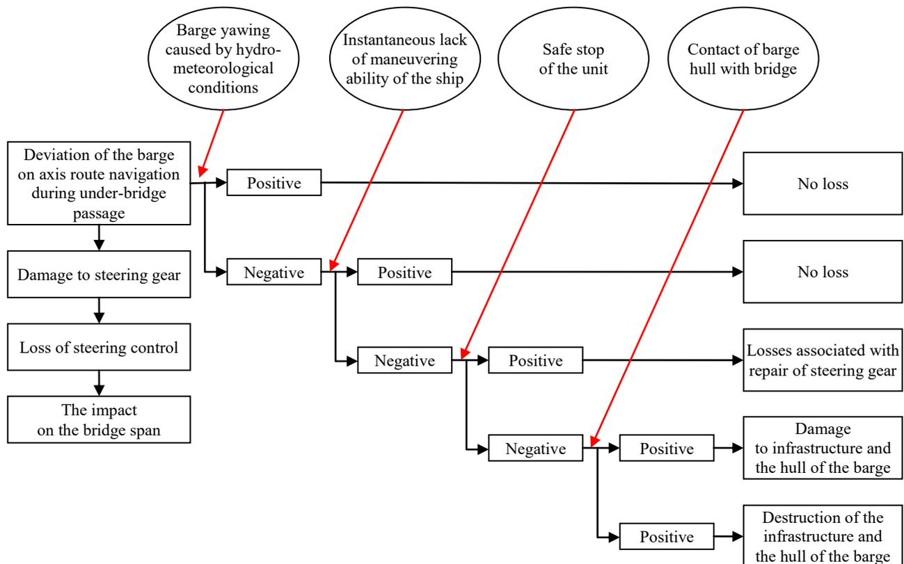
**Figure 2. Model identification of hazards during under-bridge passage by an inland vessel, built using ETA techniques**
