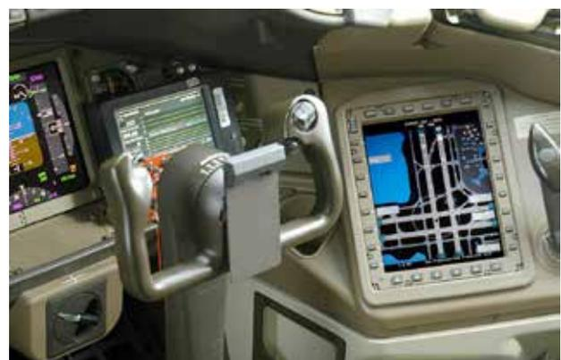
**Figure 3. Integrated “electronic flight bag” (Jeppesen, 2012)**
