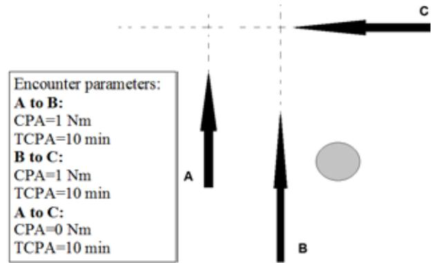
Figure 7. An example encounter situation of three ships: A, B, C
