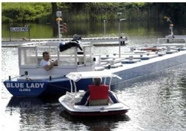
Figure 4. Manned tug working with model tanker
