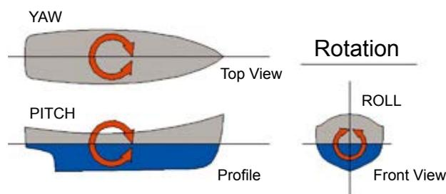
Figure 2. Rotation of coordinate systems: Pitch, Roll, Yaw – Tait-Bryan angles (Wikipedia, 2015)
