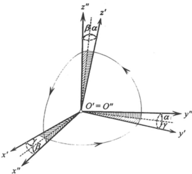
Figure 1. The orientation of spatial systems using Euler angles (Czarnecki, 2014)
