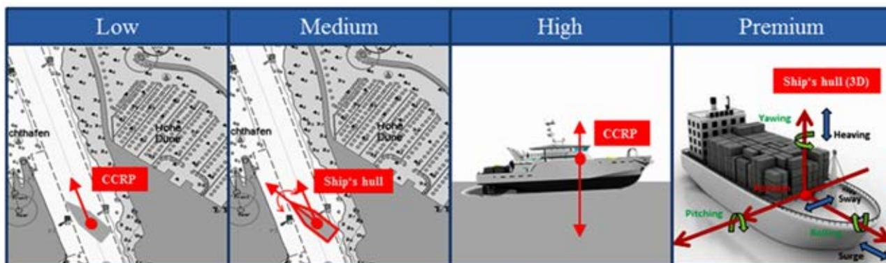
Figure 2. Proposed performance level regarding the amount and the types of onboard PNT data provision
