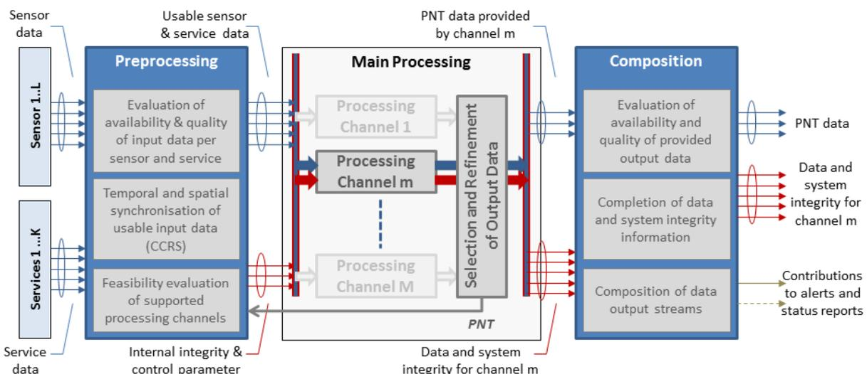
Figure 3. Generalized model of onboard PNT data processing
