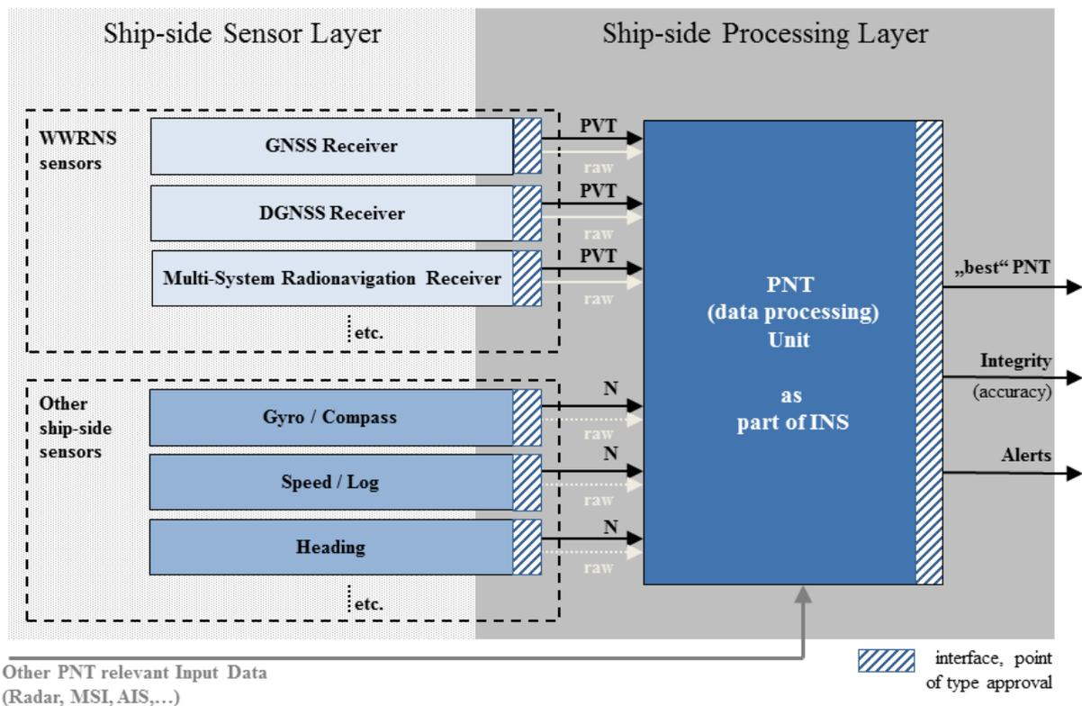
Figure 4. A PNT unit as part of MRR (top) and INS (bottom)
