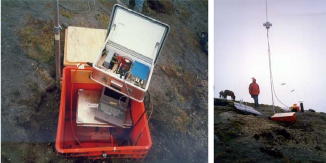
**Figure 1. The low-latency/high-rate GNSS operating station on Popocatepetl (The laptop computer is used only for maintenance. It is not a part of the station equipment)**
