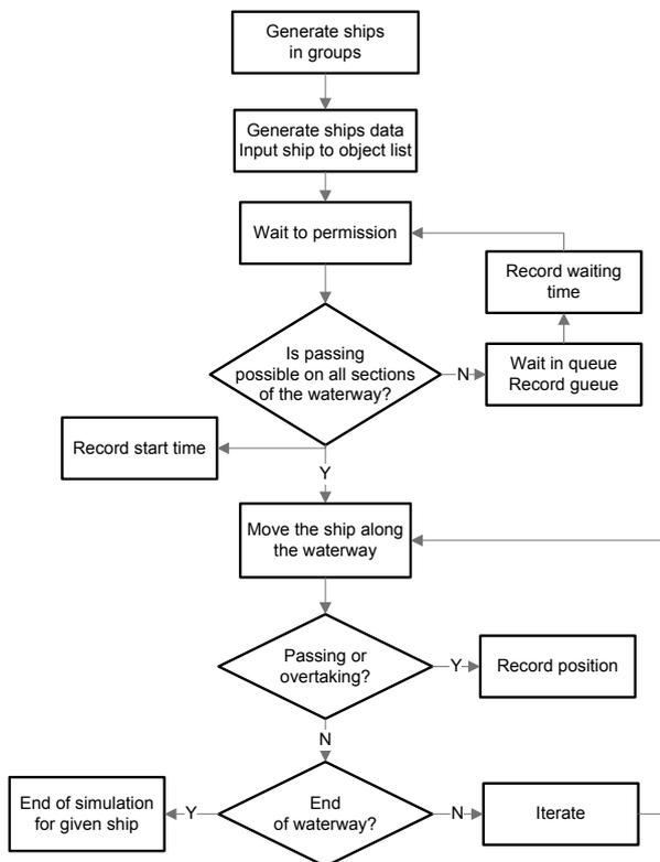
Figure 2. Stochastic microscopic simulation model of ship traffic in Świnoujście–Szczecin waterway
