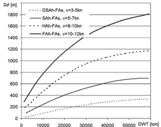
Figure 4. Stopping distance ( $S_d$ ) in case of accident of followed-by ship in step-manoevre through narrow waterway for general cargo ships (Report, 1980)
