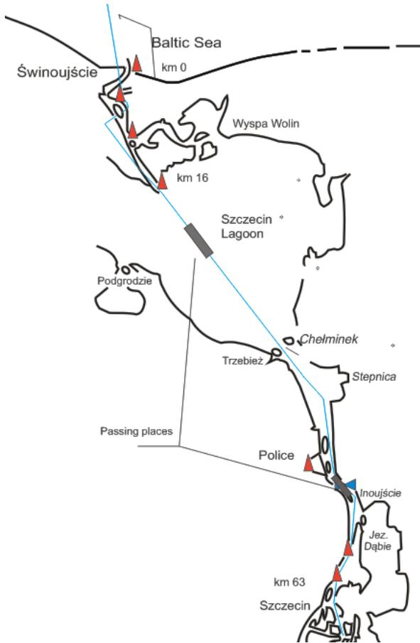
Figure 1. Layout of Świnoujście–Szczecin waterway with planned passing places for future layout
