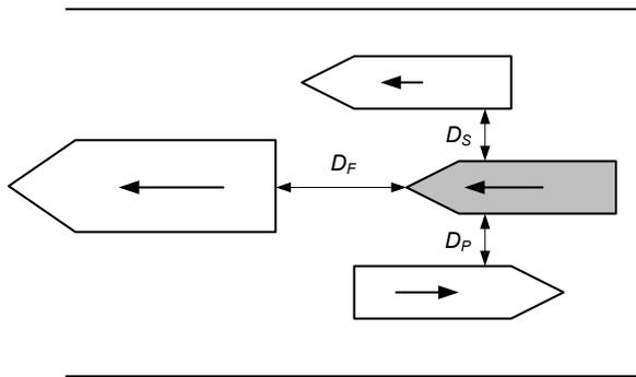
Figure 3. Ships domain parameters in narrow waterway
