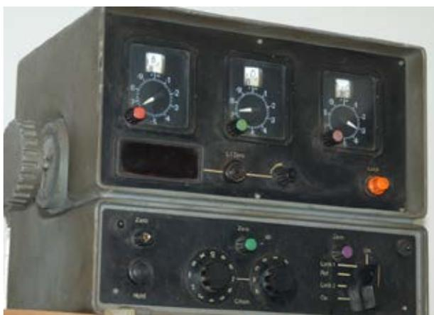
Figure 9. Decca receiver MK21 used as part of the simulator (photo by T. Budzan)
