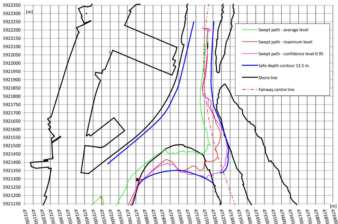
Figure 3. Variant III. Locations and manoeuvring tactics in Przesmyk Orli Turning Basin. Safe manoeuvring area of the container ship  $L_{OA} = 250$  m and navigable area (safe depth contour 12.5 m)
