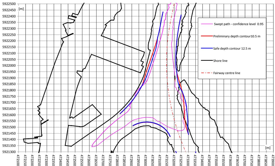
Figure 2. Variant II. Locations and manoeuvring tactics in Przesmyk Orli Turning Basin. Safe manoeuvring area of the cruise ship  $L_{OA} = 260$  m and navigable area (safe depth contour 12.5 m)
