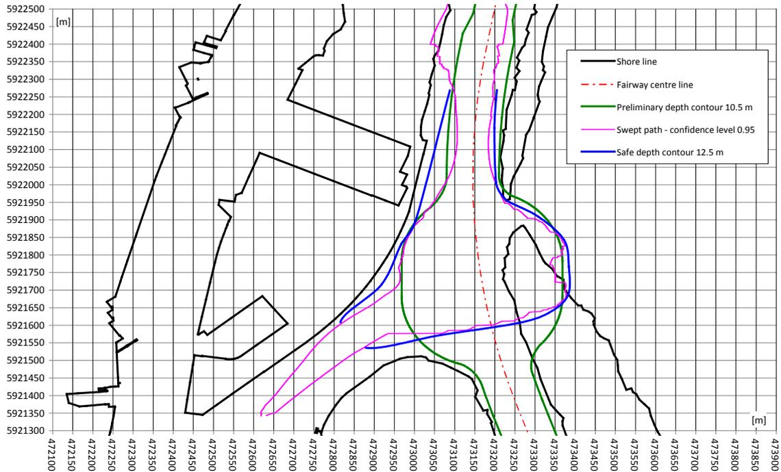
Figure 1. Variant I. Locations and manoeuvring tactics in Przesmyk Orli Turning Basin. Safe manoeuvring area of the cruise ship with  $L_{OA} = 260$  m and navigable area (safe depth contour of 12.5 m)
