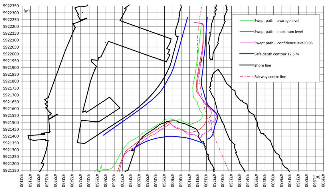
Figure 4. Variant IV. Locations and manoeuvring tactics in Przesmyk Orli Turning Basin. Safe manoeuvring area of the container ship  $L_{OA} = 250$  m and navigable area (safe depth contour 12.5 m)
