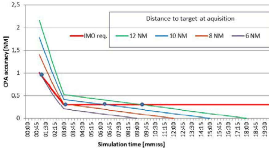
Figure 5. Calculated maximum CPA errors according to tracking target accuracy specified for CPA and relative course – Scenario 2\_1 (relative speed: 40.0 kn)
