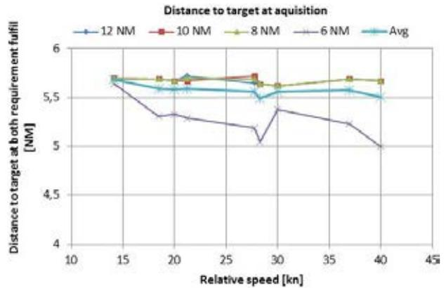
Figure 7. Distance to target when both IMO requirements are fulfilled
