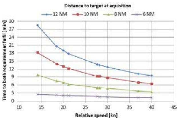
Figure 6. Tracking time when both IMO requirements are fulfilled
