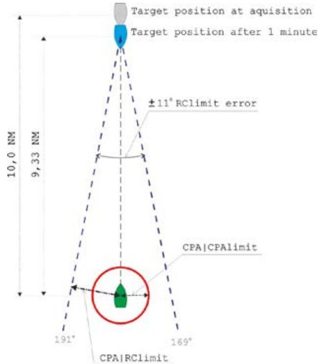
**Figure 1. Relation between CPA|CPALimit and CPA|RCLimit values (based on scenario 2\_1)**
