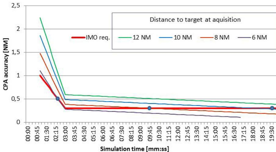
Figure 4. Calculated maximum CPA errors according to tracking target accuracy specified for CPA and relative course – Scenario 1\_3 (relative speed: 14.14 kn)
