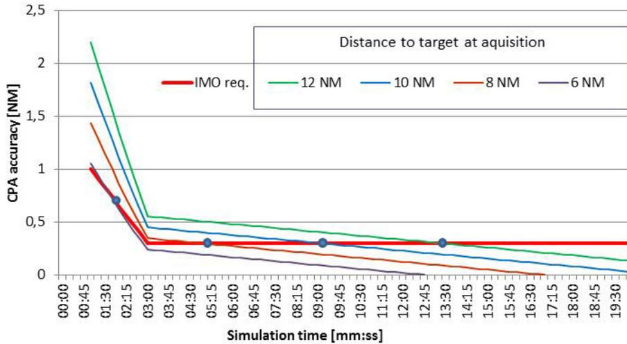
Figure 3. Calculated maximum CPA errors according to tracking target accuracy specified for CPA and relative course – Scenario 1\_1 (relative speed: 28.28 kn)
