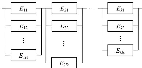
Figure 2. The scheme of a parallel-series system
