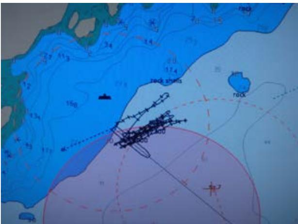
Figure 2. Screenshot from ECDIS showing the event of dragging the anchor
