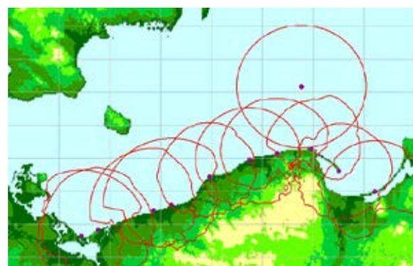
Figure 2. Areas monitored by the Polish network of the shore-based AIS stations after its modernisation and expansion (Urząd Morski w Gdyni, 2015)
