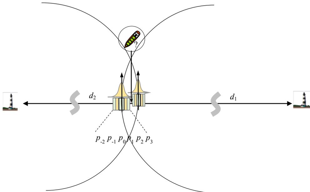
Figure 1. Graphical interpretation of two imprecise measurements, distorted with random and systematic errors, taken for objects at opposite directions
