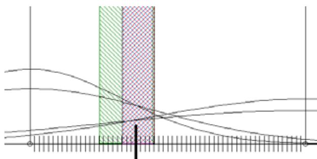
**Figure 3.** The case presented in Figure 2b with proportionally enlarged observation mean errors. Vertical shapes refer to the interval valued standard deviations with respect to the measurements
