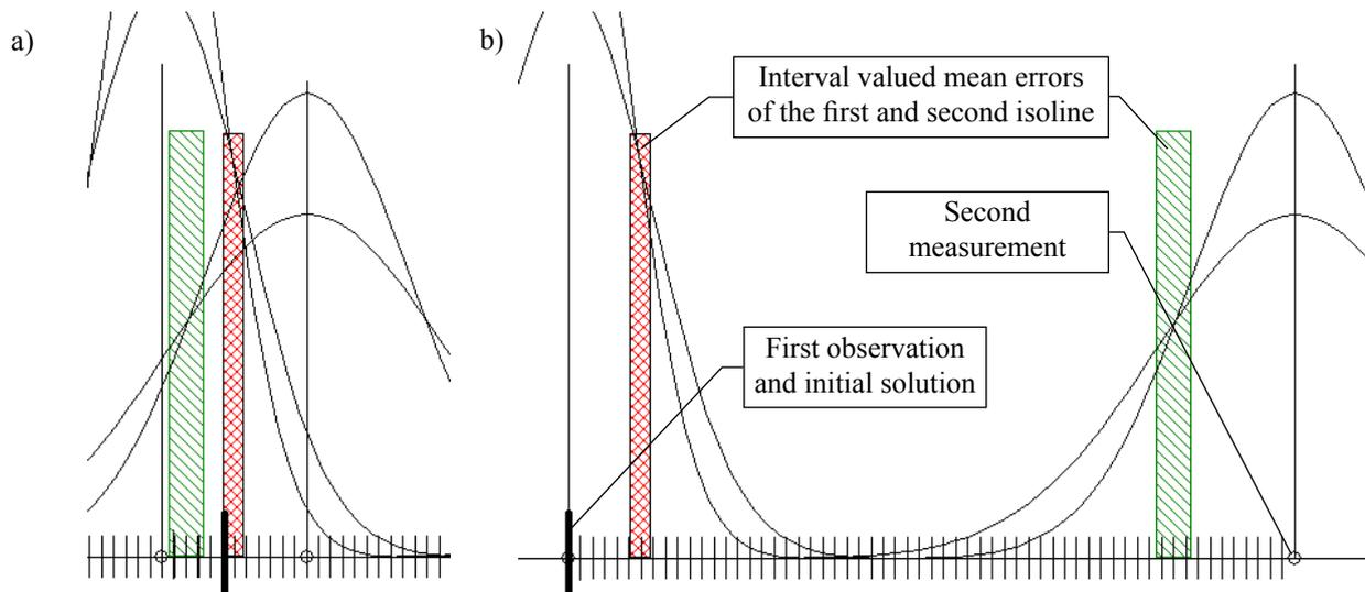
Figure 2. Two cases related to two pairs of observations made for two objects situated at opposite directions. Vertical rectangles refer to interval valued the standard deviations with respect to the measurements
