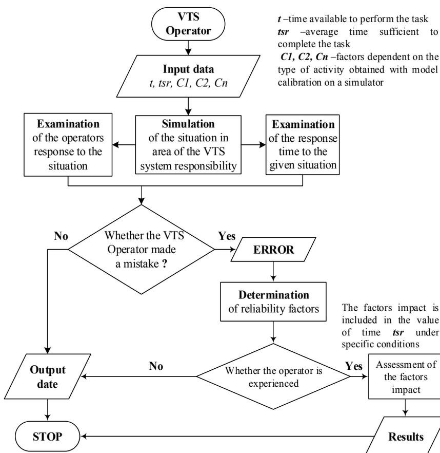
Figure 5. Block diagram of the simulation method
