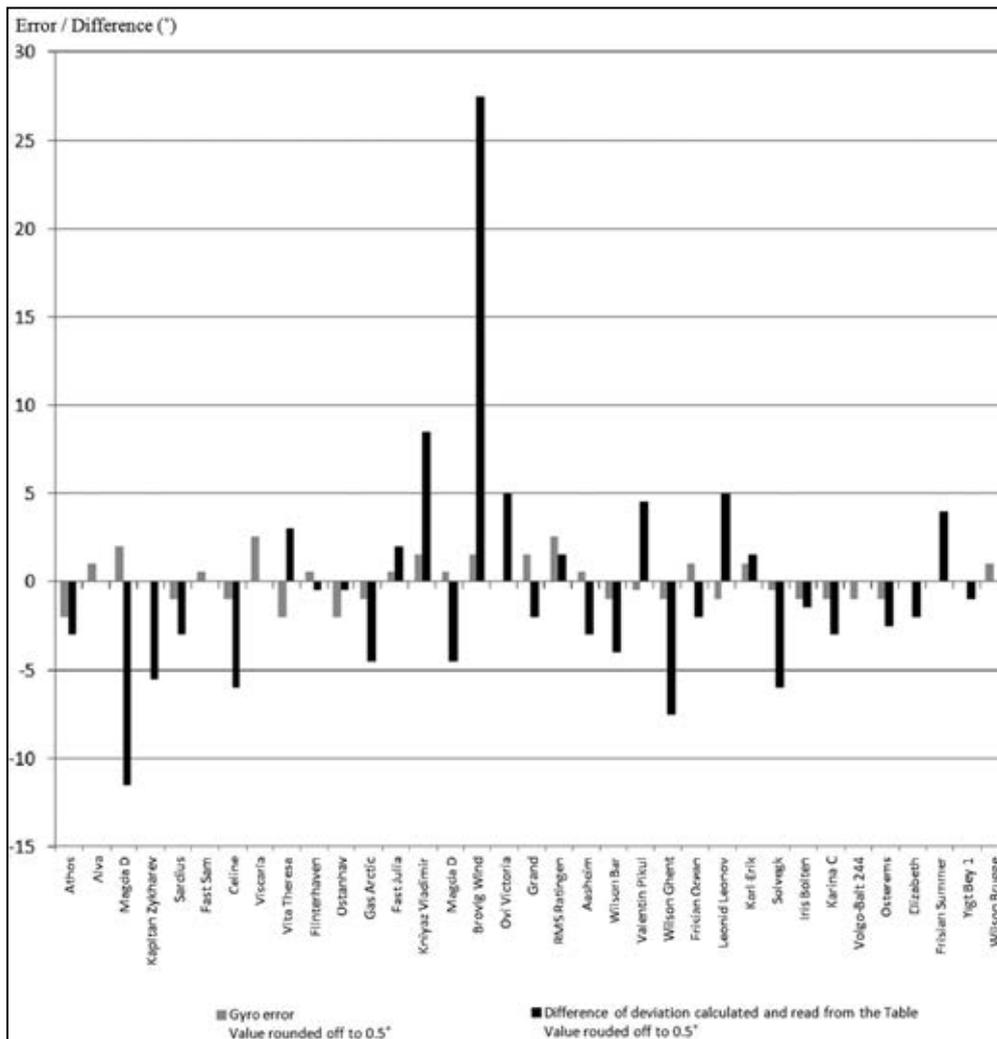
Figure 2. Results of gyrocompass and magnetic compass indication control
