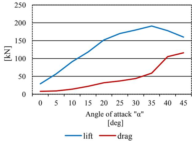
**Figure 3. Amount of drag compared to the amount of pulling power (lift) produced by B46**
