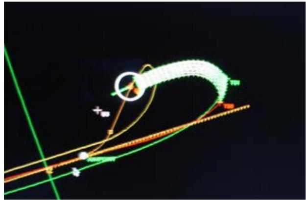
Figure 8. A real example of turn adjustment (current direction approx. 95 degrees, speed approx. 1.7 kn)
