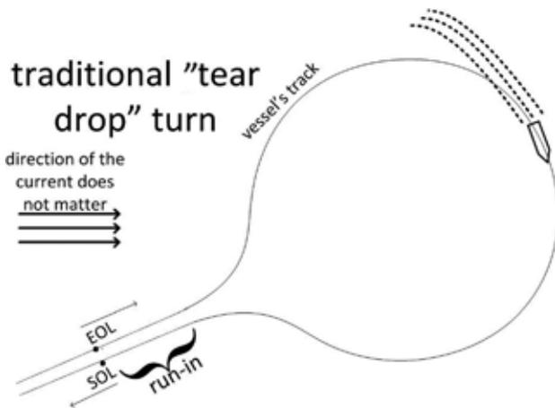
Figure 6. A traditional, unplanned turn wasting time and energy
