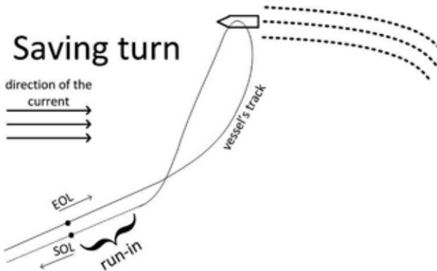
Figure 7. A preplanned turn saving time and energy
