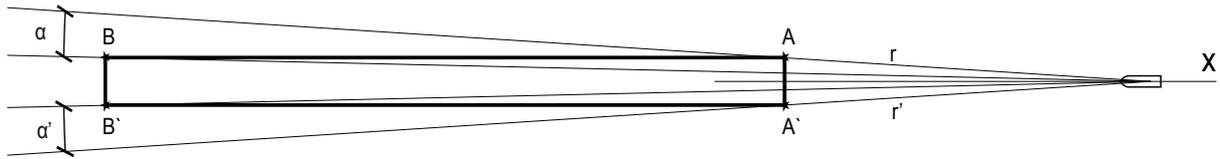
Figure 1. Mathematical model of a rectangular leading line in a radial coordinate system
