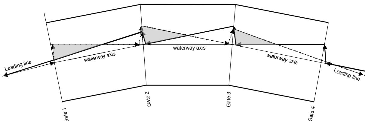
Figure 6. Schematic diagram of navigation in leading lines in the opposite directions
