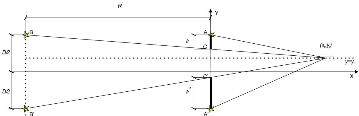
Figure 3. The use of Thales assertion in the description of a rectangular leading line in a Cartesian coordinate system
