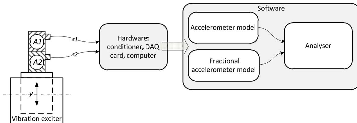
**Figure 3. Measurement system (Luft, Szychta & Pietruszczak, 2015)**
