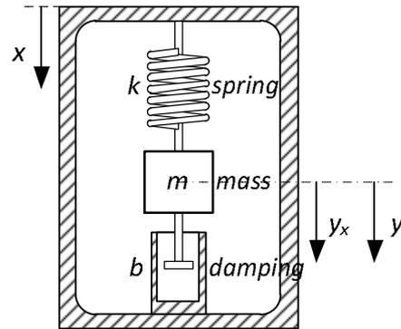
**Figure 1. Diagram of an accelerometer's design:  $x$  – object motion relative to a fixed system of coordinates,  $y$  – motion of a vibrating mass relative to a fixed system of coordinates,  $y_x$  – motion of a vibrating mass relative to a vibrating object (Luft et al., 2011; Luft, Szychta & Pietruszczak, 2015)**
