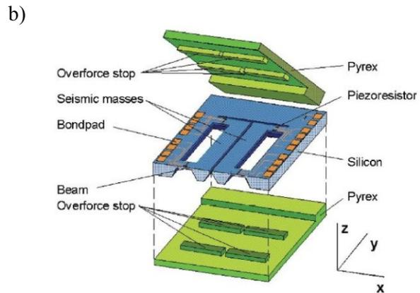
**Figure 2. Piezoelectric accelerometer: a) general design, b) design of the element for seismic mass movement conversion into electric signal (Walter, 2008)**
